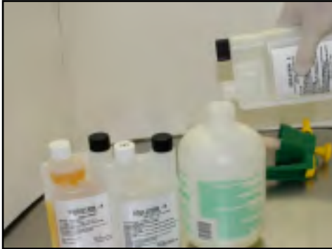
◀ Figure 6 Pour 30 ml. of Part C into the sprayer container and fill with potable water to 1 quart (32 oz.) mark.
