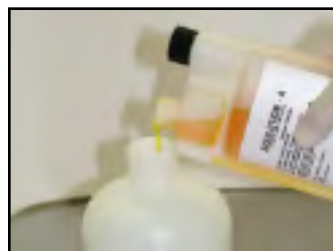
◀ Figure 3 Pour 30 ml. of Part A into 1/2 quart (16 Oz.) of potable water in a sprayer container.
