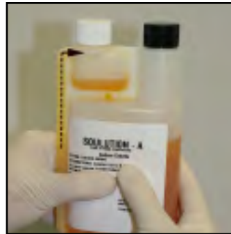
◀ Figure 1 Loosen reservoir cap and gently squeeze liquid from bottle into measuring reservoir.
